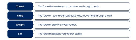
These forces are all related to each other during flight – to get a rocket off the ground, you need to increase thrust to counter its weight and drag. Then, lift keeps the rocket stable during flight.
