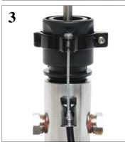
Mount assembled launcher onto the ABS base with the SS Phillips screw. Stretch out brake cable & place fat barrel nipple into the brake lever slot, thread through, and secure with silver slack adjustment ring. Insert other end of cable housing into manifold cable stop, push hose connector down & place nipple into clamp-on cable stop. Remove excess brake cable slack by ring or screwing in Phillips screw on lever. Increase or decrease brake cable slack by raising or lowering clamp-on cable stop.
